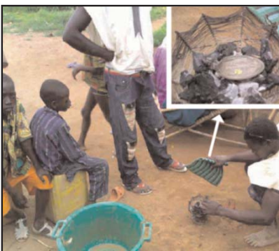
Figure 4. A man burning amalgam in front of children and in a residential area (source: UNEP, 2012)
