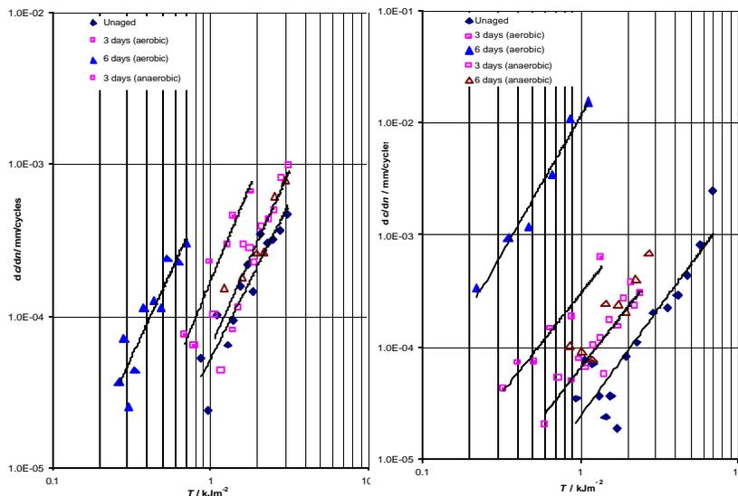
Figure 3 and figure 4: Crack growth rate ( $dc/dn$ ) as function of tearing energy ( $T$ ) for efficiently cured NR and conventionally cured NR aged aerobically and anaerobically at  $100^{\circ}\text{C}$ .
